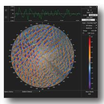
Using the *transect line* (green) feature, the operator can visusalize quiet periods to aid in equipment deployment or reclamation.
