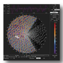
Unique *colour coding* allows the user to quickly identify extraordinary wave activity and make any necessary corrections.
