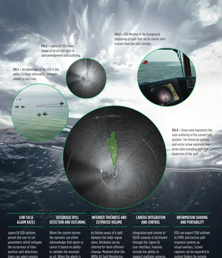
sigma S6 OSD systems permit the user to set parameters which mitigate the occurrence of false positive spill detections. Users can select regions of the scan area to ignore based on known anomalies and can also prescribe specific ranges or distances from the scanner to exclude for detection. Minimum alarm thresholds can also be set.
