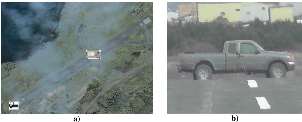
Figure 1: First scenario. a) Location of the truck and signal generator at Bell Island with a 400 meter clear range from the radar van to signal generator. b) Signal generator connected to a horn antenna in front of a truck, transmitting a reference signal 400 m away from the radar van.
