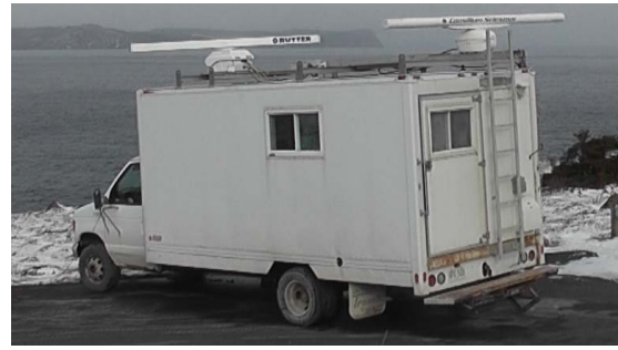
Figure 2. Rutter's mobile radar test platform equipped with the vertical and horizontal polarized radars.
