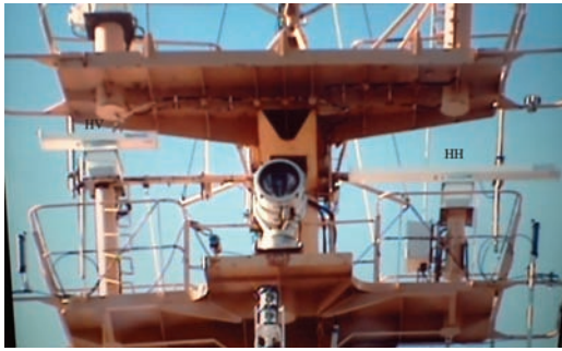
Fig. 1: (a) X-band radar system installed on the CCGS Henry Larsen which is capable of measuring co-polarized and cross-polarized radar return signal.
